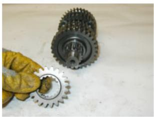
Remove the sixth speed gear and collect the washer.
