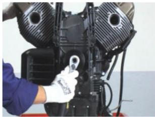
Position the generator and the timing belt.
