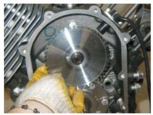
Loosen and remove the three screws and collect the washers.
