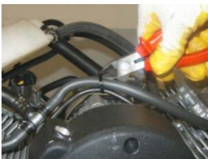
• Release the two clamps retaining the oil breather line.
