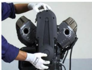
Tighten the five screws; proceed in steps and in a cross pattern.
