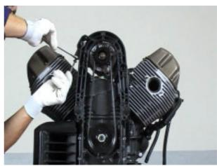
Tighten the generator retaining screws.
