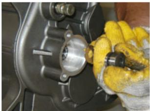
• Remove the thrust bearing and cap.
