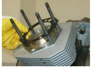
Remove the cylinder clear of the stud bolts, do not damage the piston.
