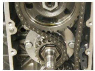
• Using the suitable tool (part no. 12.91.18.01) lock the starter gear.
