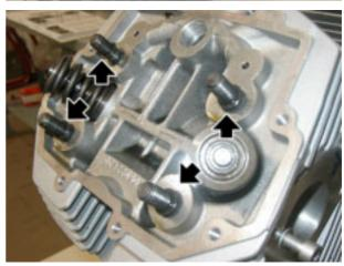
Slide out the head and collect the gasket.
