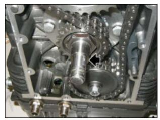
Loosen and remove the central nut securing the timing drive gear on the crankshaft and collect the washer.
