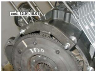
Loosen the central nut securing the camshaft gear and collect the washer.
