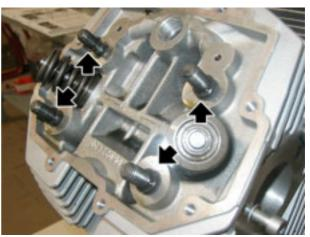
Set the two washers and tighten the two screws.
