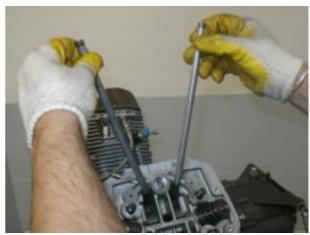
Install the rocker arm support and change the four Orings.
