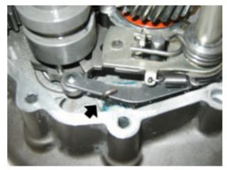
• Press on the selector to help removal of the complete transmission lever.
