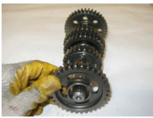
Remove the circlip.
