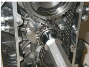
Loosen and remove the nut and collect the washer.
