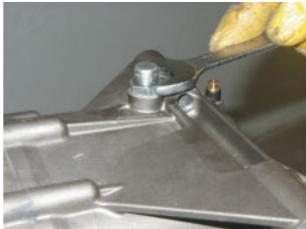
Set a suitably sized container under it, loosen and remove the plug; drain all oil from gearbox, as described in the reference chassis manual, see (REFERENCE MANUALS).
