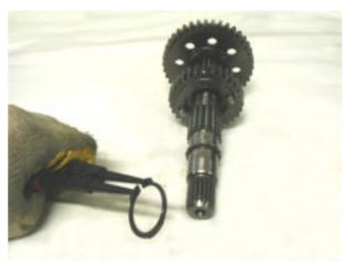
Remove the fifth speed gear.
