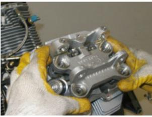
• Slide out the two rocker arm rods
