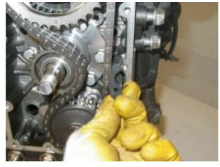
Slide out the pick-up ring and collect the dowel.
