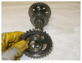
Remove the circlip.
