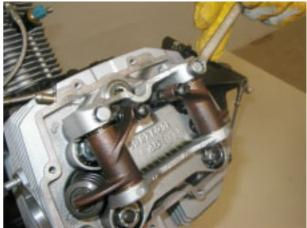
Remove the rocker arm shafts.
