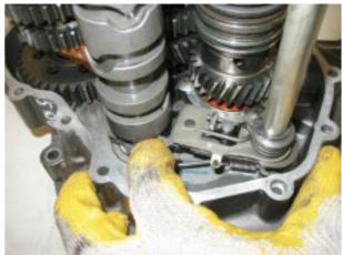
Loosen and remove the reference threaded pin.
