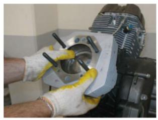
• Fit the gasket at cylinder base.
