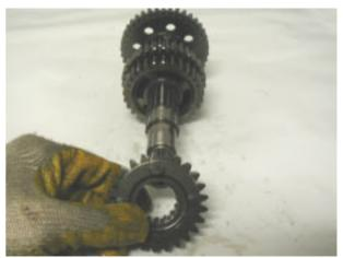
• Remove the circlip and collect the washer.
