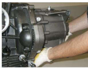
• Set the gearbox on the suitable gearbox support (part no. 14.92.96.00) and in a vice.
