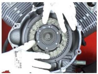
Position the gear wheel aligning the reference mark to the flywheel one.
