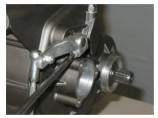
Loosen and remove the plug.
