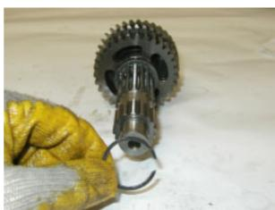
Remove the fifth speed gear and collect the roller cage.
