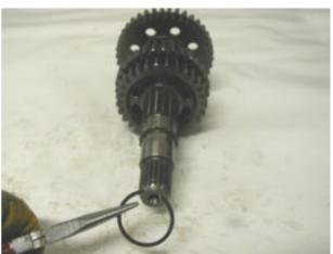
Remove the fourth speed gear and collect the roller cage.
