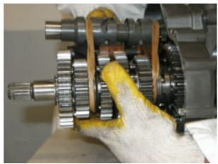
Remove the bearings from the gearbox.
