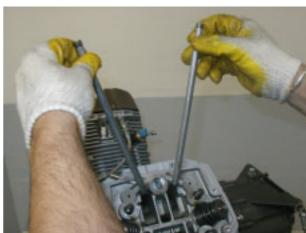
Using the suitable special tool (part no. 05.90.19.30), loosen and remove the internal spark plug.
