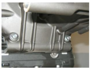
Unscrew and remove the screw.
