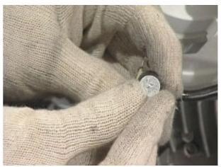
• Position the sensor to the timing cover and take it against the pick-up ring.
