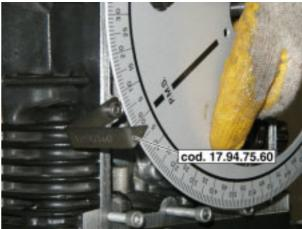
• Fit a dial gauge support to left cylinder external spark plug, and fit a dial gauge on the support.
