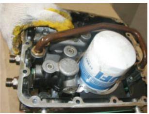
Once these parts are removed, it is possible to gain access to the oil pressure control valve and the thermostatic valve. Remove them, if necessary.
