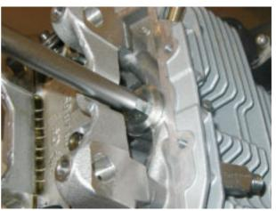
Connect the line delivering oil to the head and tighten
