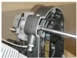
Remove the belt and the generator complete with pulley.
