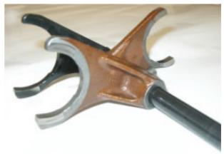
Slide out the forks and collect the shaft.
