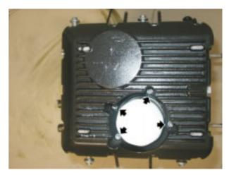
Release and remove the two screws.
