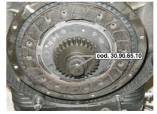
Loosen and remove the eight screws securing the flywheel gear wheel.
