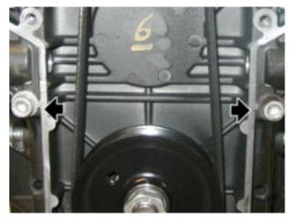
Loosen the nut and collect the screw.
