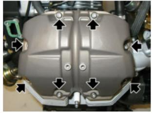
Remove the head cover and collect the gasket.
