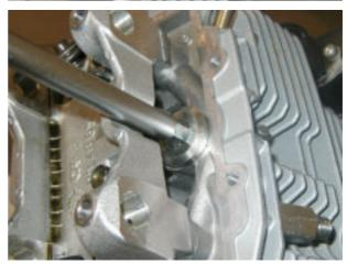
Loosen and remove the socket nut and collect the washer.
