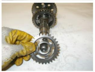
Remove the third speed gear and collect the roller cage and the washer.
