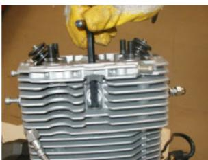
Using the suitable special tool (part no. 05.90.19.30), tighten the internal spark plug.
