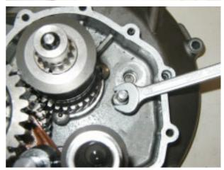
Use elastic bands to tie the gearbox shafts and remove the unit.
