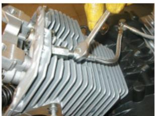
Loosen and remove the threaded plug.
