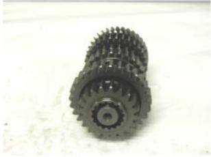
Remove the second speed gear, collect the roller cage.
