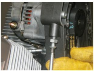
• Completely unscrew and remove the screw.
