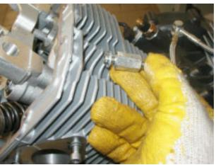
Loosen and remove the four nuts and collect the relevant washers.
