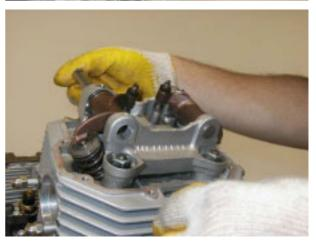
• Remove the rocker arm and collect the three washers.
