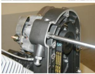
Loosen the nut and release the adjuster, so that generator can slide down.
