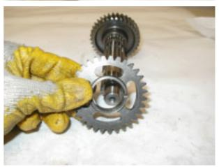
Using a suitable heater, heat up the shaft and remove the transmission helical gear.
