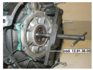
Slide the crankshaft from the back.
