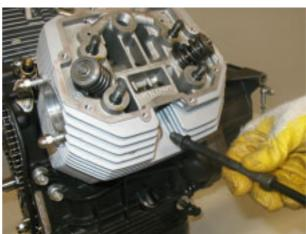
Slightly detach the head from the cylinder and remove the four O-rings.
