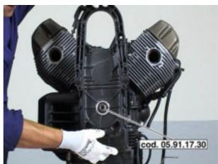
• Tighten the two screws.
