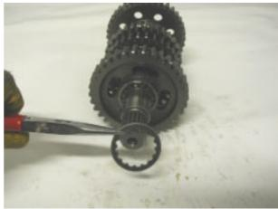
Remove the second speed gear and collect the roller cage and the washer.
