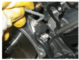
Fit a suitable flat washer on the sensor, measure its thickness.
