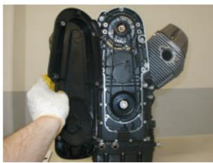
Release and remove the eight screws.
