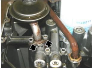
• Remove the black flange and collect the seal.
