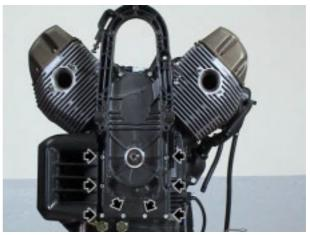
Tighten the ten screws; proceed in steps and in a cross pattern.
