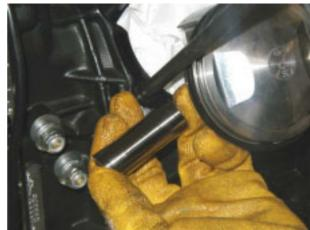
Fit gudgeon pin circlip.
