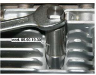
Loosen and remove the two screws and collect the two washers.
