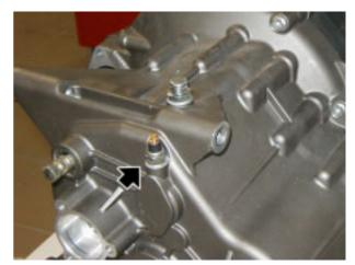
Slide out the cylinder and collect the O-ring and the washer
