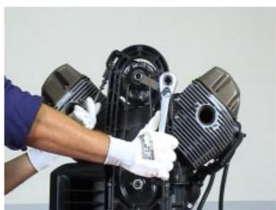
Tighten the lock nut.
