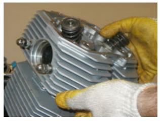
Fit the special tool (part no. 10.90.72.00) to top retainer and at the centre of the valve to be removed.
