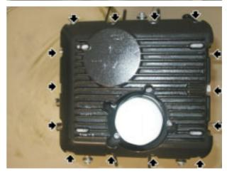
Loosen and remove the four screws and remove the black oil sump.
