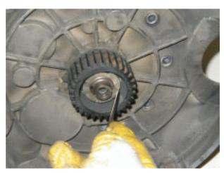
Using the suitable pin wrench (part no. 05.91.26.30) and clutch locking tool (part no. 30.91.28.10), loosen and remove the ring nut; collect the inner clutch body.
