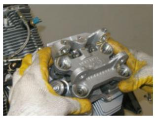
• Fit the four washers and tighten the four nuts.
