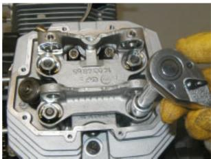
Install the washer and tighten the socket nut.
